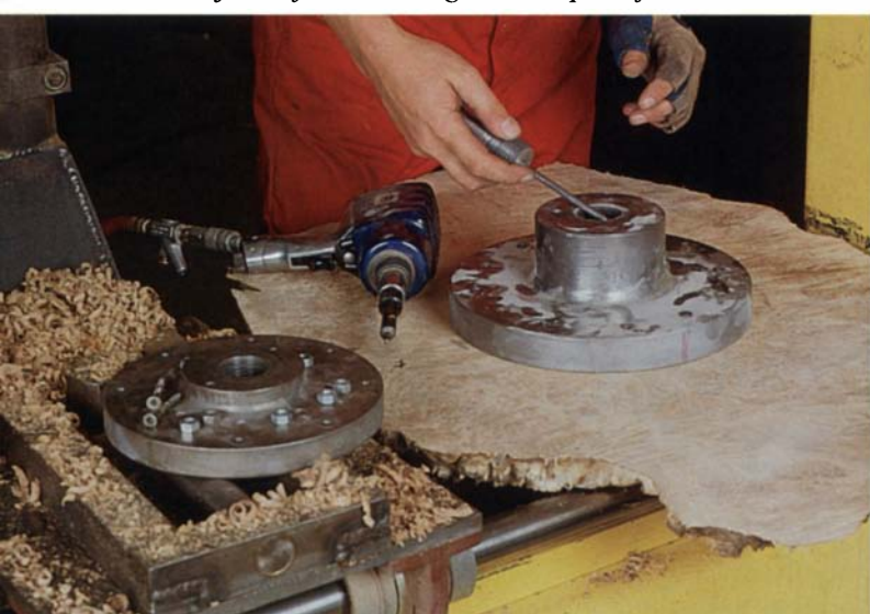
Below: The author has removed the faceplate from the front of the slab and has mounted a larger faceplate on the back side after turning it true. The aluminum bar with the pointed rod is used to center the faceplate on an indentation that was made with the tailstock center just before removing the workpiece from the headstock.
