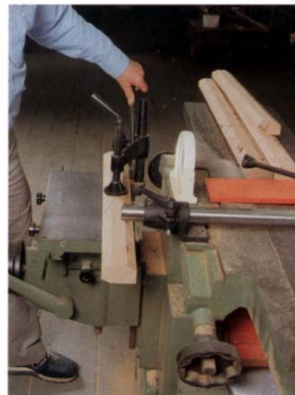
Bed rails can be joined to posts with standard metal bed hardware, mortised into both the rail ends and the posts. After fitting the hardware into its shallow mortise in the post, McAlevey marks where secondary mortises must be cut to accept the books on the mating hardware (left). He mills mortises with a Steton combination machine (right). The round mirror mounted on top of the machine enables him to line up the stock with the cutter without having to crane over the workpiece.
