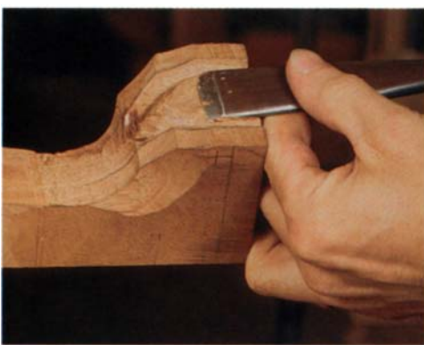
Above: Headley shapes the lower surface of the ball with a 1 1/4-in.-wide #5 gouge, powering the cut with his right hand and guiding it with his left. Right: The author carves across transitional grain at the ball's greatest diameter. The leg is held at a comfortable height and angle in an auxiliary clamp secured in the bench vise.
