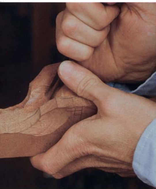
Above: The edge of the web is cut with a 1/2-in.-wide #5 gouge. Below: The concave web is cut with a 1/2-in.-wide #5 gouge.
