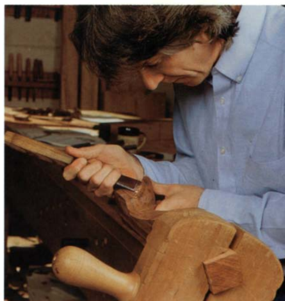
Above: Headley shapes the lower surface of the ball with a 1 1/4-in.-wide #5 gouge, powering the cut with his right hand and guiding it with his left. Right: The author carves across transitional grain at the ball's greatest diameter. The leg is held at a comfortable height and angle in an auxiliary clamp secured in the bench vise.
