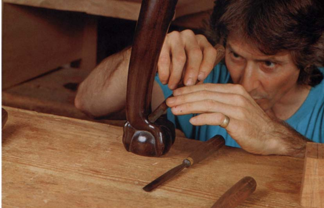
Matching the sweep and width of a 1/2-in.-wide #5 gouge to the original leg (above), Headley cuts the transition from the toe to the ankle accurately (below, left). The outside of the side toe has been scalloped to angle it toward the center toe, forcing the claw to rake back. After marking their width, the toes are roughed out with a parting tool (below, right).
