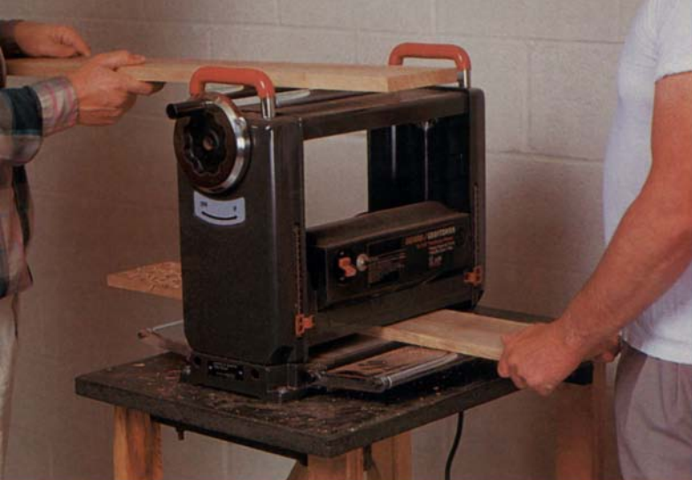
To make planing a pile of boards easier, the Dayton 6Z960 and Sears 12½ in., shown here, have top-mounted rollers to allow feeding boards over the unit on subsequent passes.
