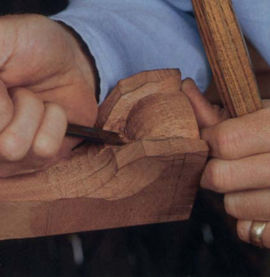
Above: The edge of the web is cut with a 1/2-in.-wide #5 gouge. Below: The concave web is cut with a 1/2-in.-wide #5 gouge.
