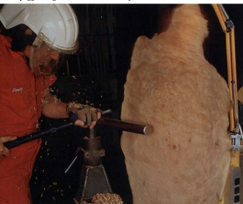
Below: The author has removed the faceplate from the front of the slab and has mounted a larger faceplate on the back side after turning it true. The aluminum bar with the pointed rod is used to center the faceplate on an indentation that was made with the tailstock center just before removing the workpiece from the headstock.
