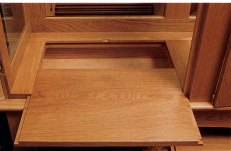
A hidden compartment at the bottom of the case is covered with a sliding door. The door frame is laminated from two pieces after a rabbet is routed along the inside edge of the top frame. A piece of hardwood veneer glued to the lower frame minimizes wear and raises the door about \frac{1}{32} in.
