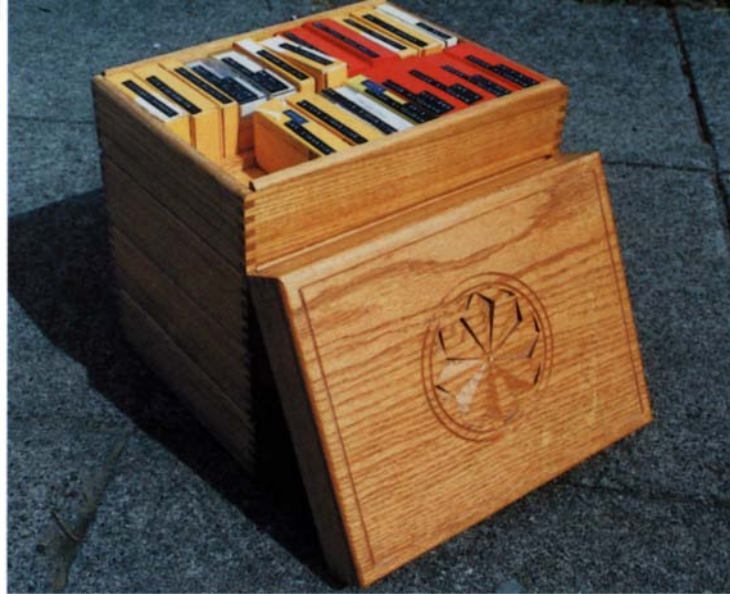
This nest of trays for slides is quarter-sawn oak with finger-jointed corners that were made on the tablesaw with a simple jig. By increasing the height \frac{1}{4} in., the trays will accommodate audio tapes.
