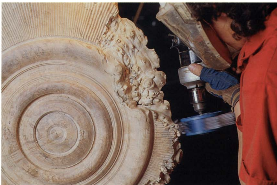
Left: The radiating lines of the carved V-grooves are laid out by rotating the workpiece in small increments and drawing along the tool rest.
