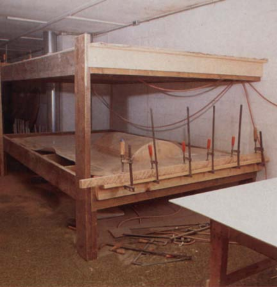
Above: This two-tier vacuum-bag setup, with a 4-ft. by 8-ft. bag on top and a 5-ft. by 10-ft. bag below, doubles the author's veneering capacity. Clamps and battens seal the bag and a mercury switch on the wall maintains a constant vacuum. Right: The VacuPress can be set up easily and disassembled quickly. Ideal for the small shop with limited production, the quality and durability of this unit make it equally suited to full-time veneering operations.
