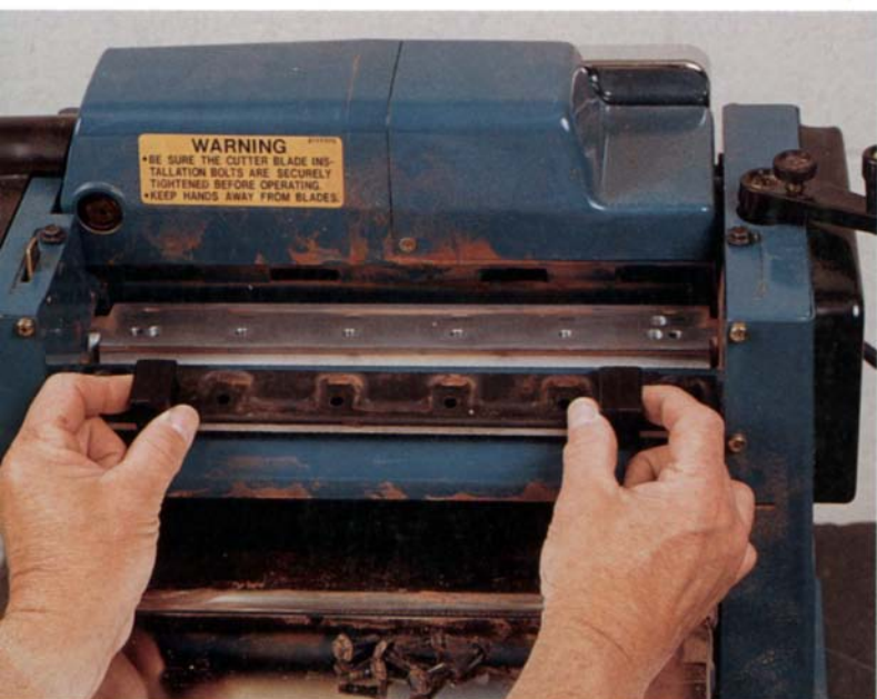
To make changing knives easy and fast, the Makita 2012 employs a system including a spring-loaded lock to fix the cutterhead, reversible, disposable knives, and a pair of magnetic handles, shown in use here. These are all designed to help you align the knife and its holder during knife removal and replacement.
