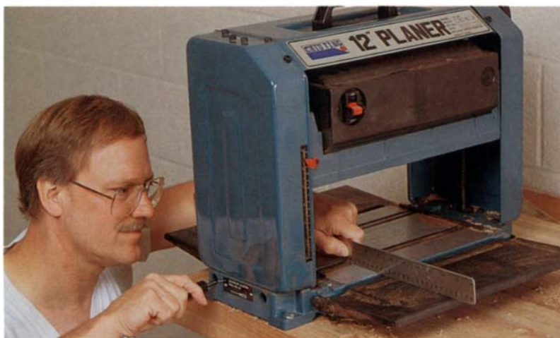
Several Taiwanese models, including the Chiu Ting CT-318 shown here, employ bed rollers, which can help green or rough stock move through the planer smoothly. Keeping the rollers at just the right height, a few thousandths of an inch higher than the bed, is a simple adjustment made with a screwdriver and a straightedge.
