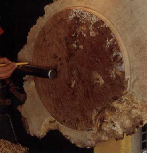
Left: The radiating lines of the carved V-grooves are laid out by rotating the workpiece in small increments and drawing along the tool rest.
