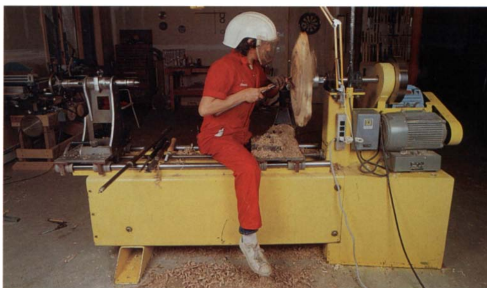
Elliott sits astride the custom-made lathe that makes it possible for him to turn these large irregular pieces. In spite of its size, the lathe can be made portable by unbolting the bed portion from the headstock. After the lathe is assembled, the base can be filled with sand, which increases its weight to 3,000 lbs.
