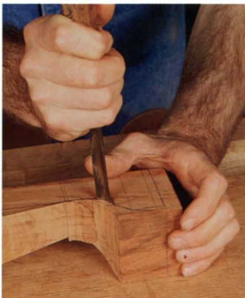
Matching the sweep and width of a 1/2-in.-wide #5 gouge to the original leg (above), Headley cuts the transition from the toe to the ankle accurately (below, left). The outside of the side toe has been scalloped to angle it toward the center toe, forcing the claw to rake back. After marking their width, the toes are roughed out with a parting tool (below, right).
