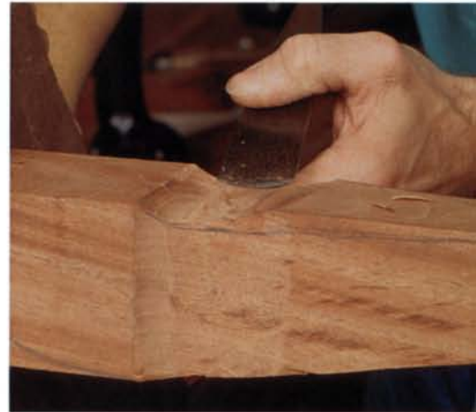
Above: Following an original discarded example, the author ripped from the knee to the ankle with a handsaw, and then he finished by cutting across the ankle with a bowsaw. Below: Headley uses a gouge to cut the shape inside the knee.
