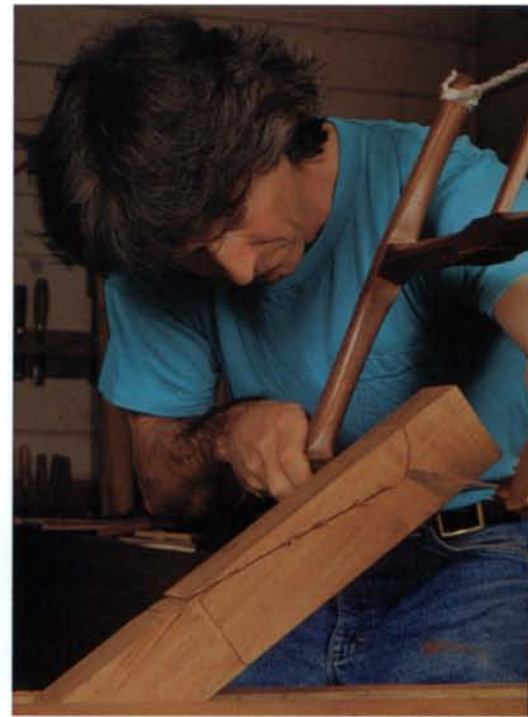
Above: Following an original discarded example, the author ripped from the knee to the ankle with a handsaw, and then he finished by cutting across the ankle with a bowsaw. Below: Headley uses a gouge to cut the shape inside the knee.
