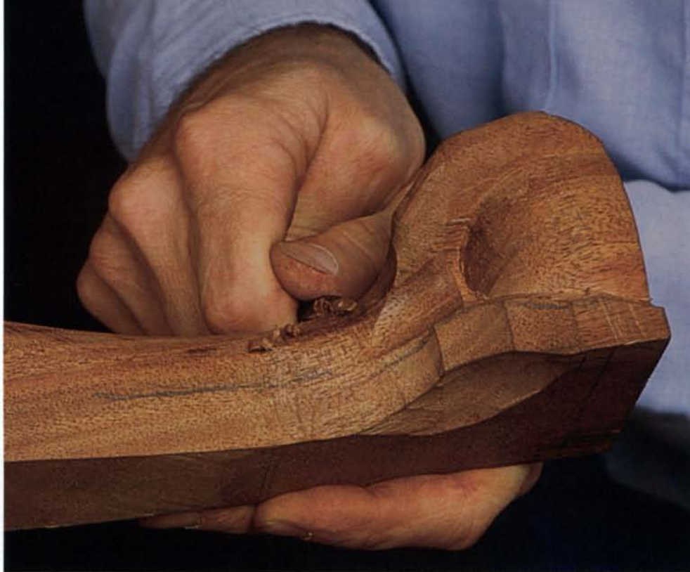
Above: Headley uses a knife to finish-carve the quick sweep of the top of the toe to the ankle. The ankle's curve gives the leg a sense of weight. Below: The shape of the rear toe and claw lends a distinctive character to the Scott ball-and-claw foot. The original leg is on the left.
