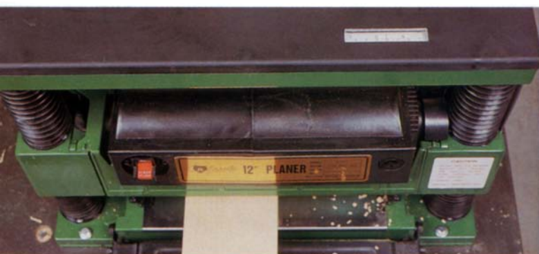
A planer is capable of accurately planing stock to a desired thickness. In lieu of a standard scale and pointer for setting the cut, the Grizzly G1017 employs a measuring tape, with markings down to 1/32 in., that shows thickness of cut through a plastic window mounted conveniently on top of the unit.
