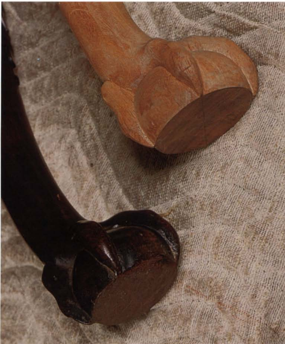
Above: Headley uses a knife to finish-carve the quick sweep of the top of the toe to the ankle. The ankle's curve gives the leg a sense of weight. Below: The shape of the rear toe and claw lends a distinctive character to the Scott ball-and-claw foot. The original leg is on the left.
