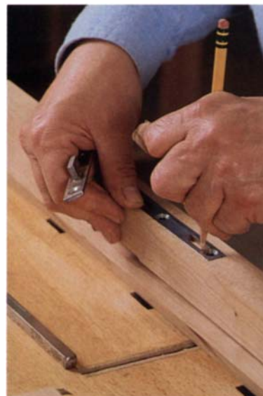
Bed rails can be joined to posts with standard metal bed hardware, mortised into both the rail ends and the posts. After fitting the hardware into its shallow mortise in the post, McAlevey marks where secondary mortises must be cut to accept the books on the mating hardware (left). He mills mortises with a Steton combination machine (right). The round mirror mounted on top of the machine enables him to line up the stock with the cutter without having to crane over the workpiece.
