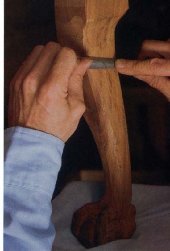
Drawing its teeth perpendicular to the stroke, a mill file leaves the leg ready to be scraped and polished.
