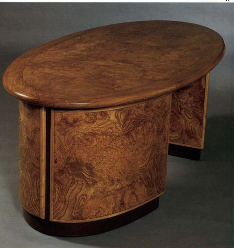
A vacuum-bag veneer press makes it easy to laminate large flat surfaces, like this desktop made by Merrick. Shaping and laminating its curved pedestals was also greatly simplified.
