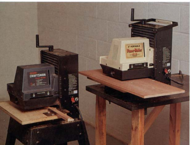
While they may only sport 6-in.-long knives, the open-sided design of the Sears Craftsman Planer/Molder, left, and the Foley-Belsaw 455, right, allows some interesting possibilities. Boards up to 12 in. wide may be planed in two passes and, with the optional molding cutters installed, these planers are capable of producing over a dozen different profiles, including this picture-frame molding being cut by the Sears model.
