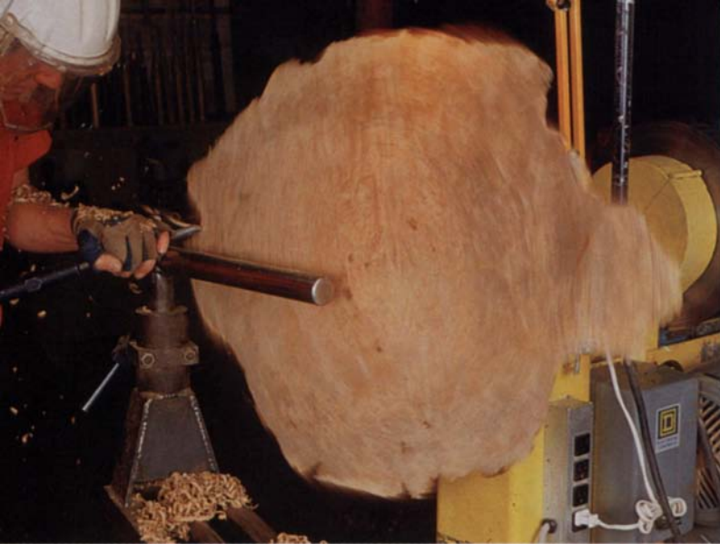
With a faceplate mounted on what will be the front of the sculpture (above), Elliott cleans up the slab's back side. It takes concentration and a steady hand braced against the tool rest to keep the tool's cutting edge in the same plane while the spinning slab's jagged edge moves in and out of contact with the tool (below).
